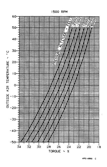
Figure 1. Propeller Low Pitch Stop (Sheet 1 of 3)
